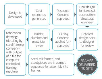
Plumbers and electricians should be involved before the frames are produced. The punching of service holes can be made during the roll-forming process, reducing time on site.
